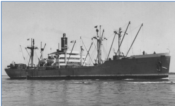
ss. Salatiga-(VC2-S-AP2), 6000pk turbine van Westinghouse Electric, 15kn.
