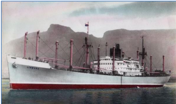
ss. Limburg (C 3 -S-A 5 ), 8500 pk turbine van Westinghouse Electric, 16,5 kn.
