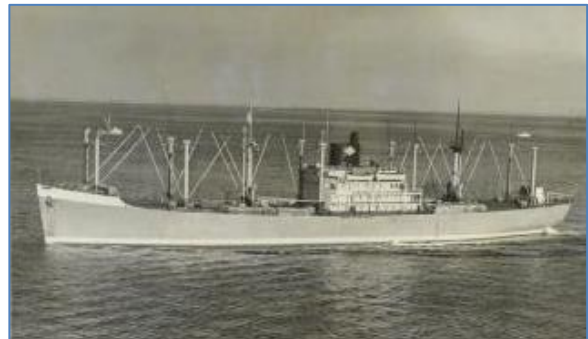
ss. Utrecht (C 3 -S-A 5 ), 8500pk turbine van Westinghouse Electric, 16,5 kn.
