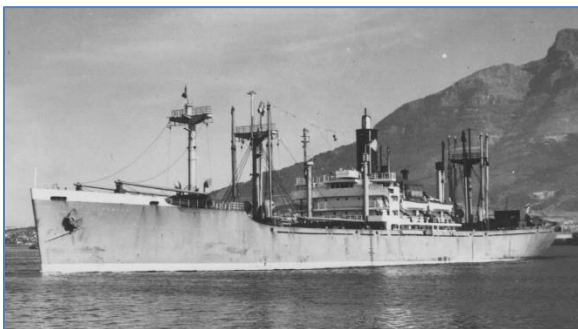
ss. Sarangan-(VC2-S-AP2), 6000pk turbine van Westinghouse Electric, 15kn.
