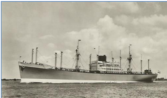
ss. Zeeland (C 3 -S-A 5 ), 8500pk turbine van General Electric, 16,5 kn.
